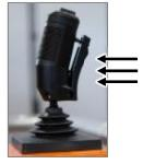
PRESS THE DEAD MAN BUTTON ON THE JOYSTICK, then move the joystick in the required direction.
