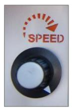
When the machine is in transport position (cage fully lowered) it is possible to regulate the transmission speed from the regulator.
